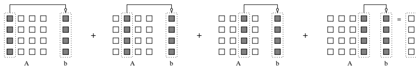
(a) Column major data access
